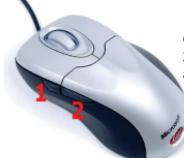
1 = Advance cutter 1 position in the active cutter path.
