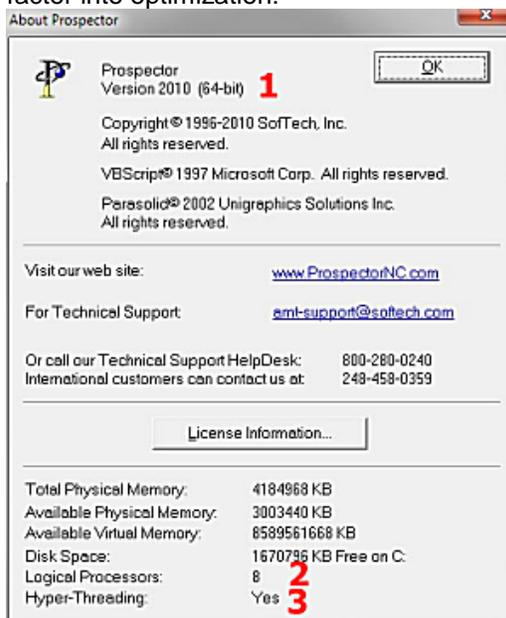
1. Version shows which edition of Prospector you have installed (32-bit or 64-bit). The 64-bit version is capable of using much more memory. More about 64-bit computing later.
