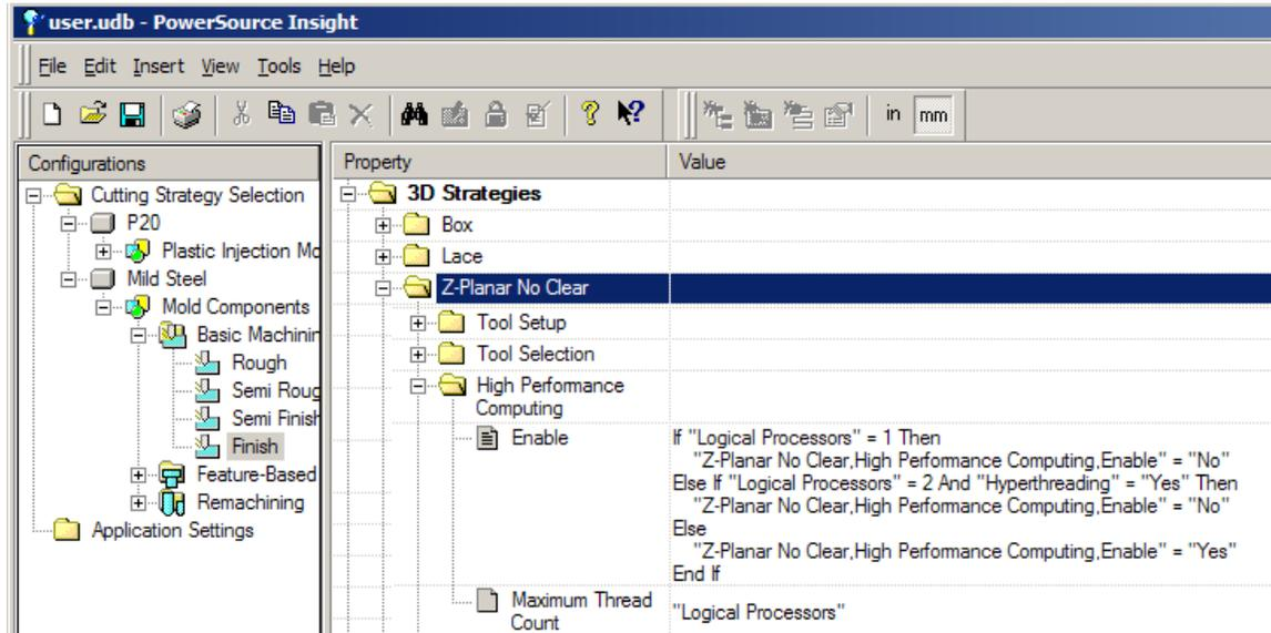
In the High Performance Computing folder, the Enable setting turns HPC on or off. The default rule is to turn off HPC if your computer has only 1 logical processor (HPC makes no sense in this case) or if your computer has 2 logical processors and has Hyper Threading (i.e. 1 physical processor with Hyper Threading such as a Pentium 4 processor). For all other cases, HPC is enabled.
